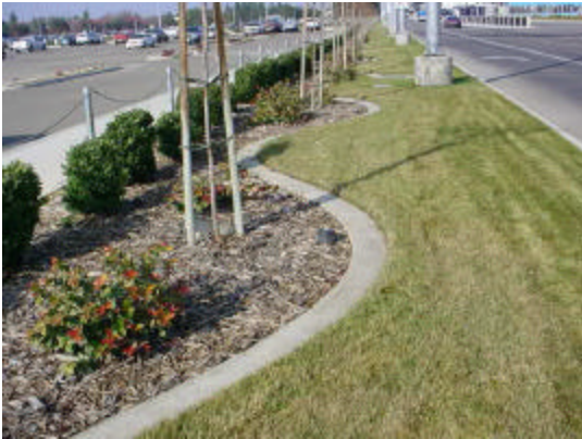
Photos I-3 (Left) and I-4 (Right). Landscape features, Examples 1 (Fresno, CA) and 2 (Sanger, CA). Edging set flush with the ground to enable mowing. Plants are drought tolerant and low maintenance. Low maintenance vegetative area has weed barrier fabric and mulch to prevent weed growth. Irrigation devices are hidden in vegetation (2.7.3.4)
