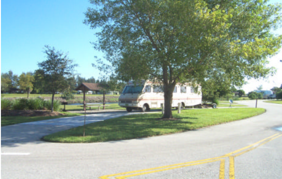
Photo M-11. Pull-through site - double. Ortona South Campground, Lake Okeechobee Waterway, FL. Note landscape plantings for buffer and aesthetics are indigeneous, low-maintenance, sustainable. Shade provided by combination of trees and shelter (Table 5.1)
