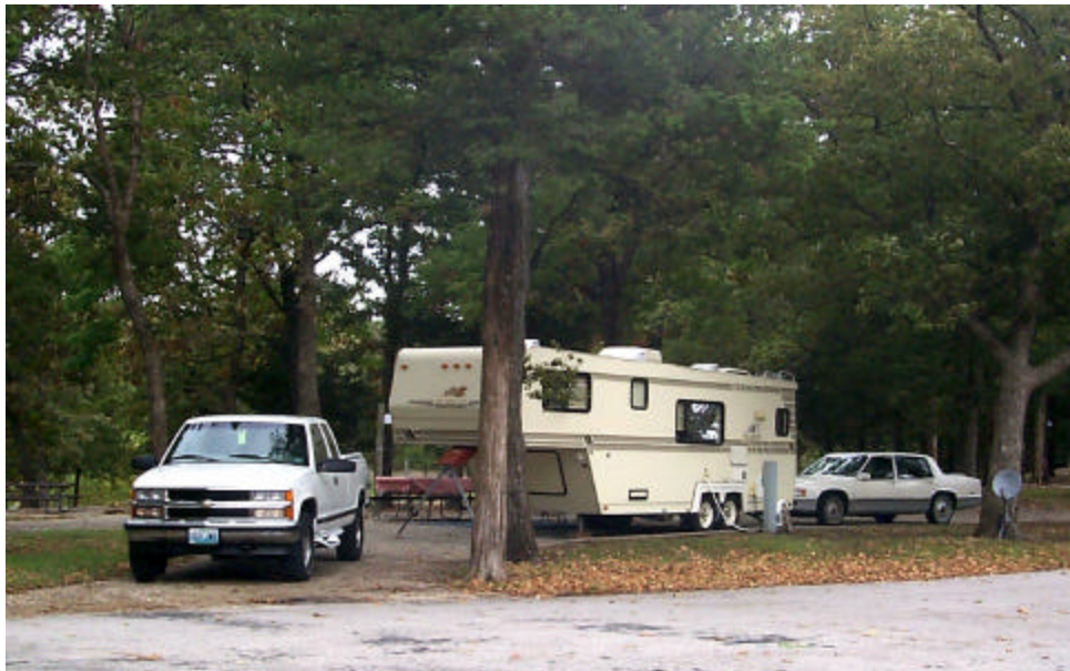
Photo M-10. Pull-through site - multiple vehicles. Pomme de Terre Lake, MO. This shaded campsite demonstrates 70-ft parking area length with room for extra vehicle, level and hardened parking area, and individual utility hookups (Tables 5.2 and 5.3)
